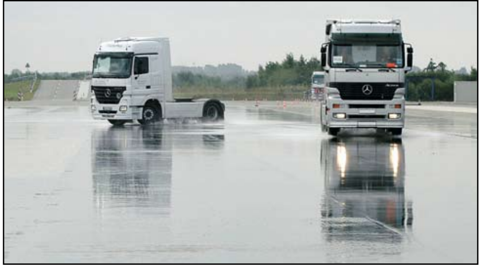
Two Mercedes-Benz trucks on a test track. The truck on the left does not have ESP and spins out of control while braking on a wet track.
