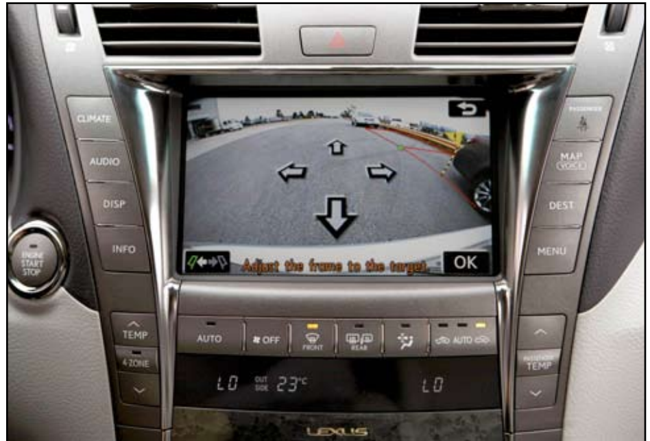
The Lexus LS 460's parking-assist system automatically steers the vehicle into a parallel or slot parking stall.
