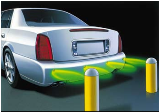
An ultrasonic rear obstacle-detection system warns the driver of obstacles behind the vehicle.
