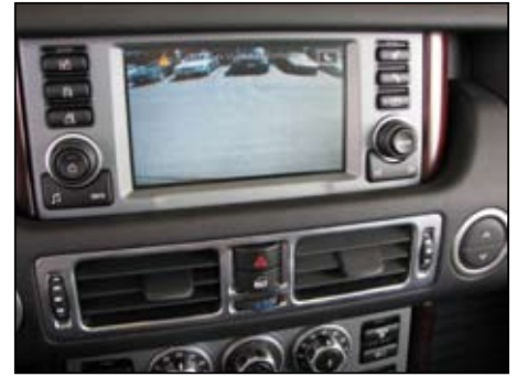
A camera system relays an image of the area behind the vehicle to a dash-mounted screen.
